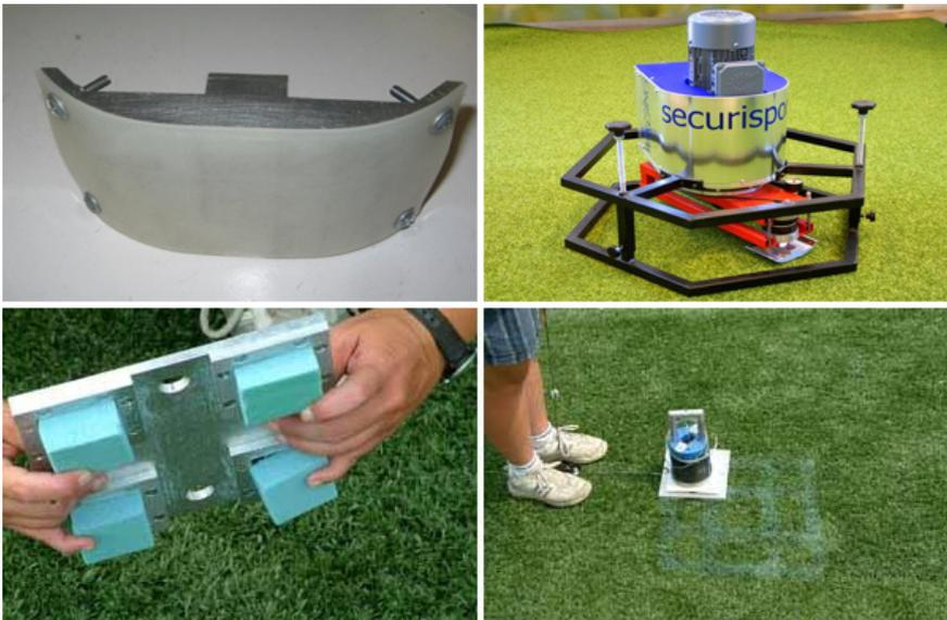
**Figure 6** Test foot and apparatus according to the FIFA method 8 (above) and foam block configuration and experimental setup of the ASTM F1015 method (under).<sup>35,39</sup>
